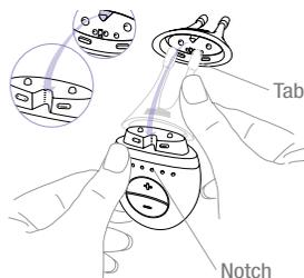
Figure 6. Align the tab to the notch for setup.
